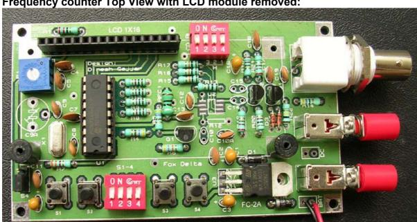
Frequency counter Top View with LCD module removed:
