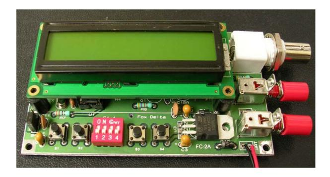
This Frequency counter Project is based on PIC16F84A Micro controller chip manufactured by Microchip. Although rated at 1.1GHZ due to Pre-Scale IC capability, it can measure up to 400MHZ in this project.
