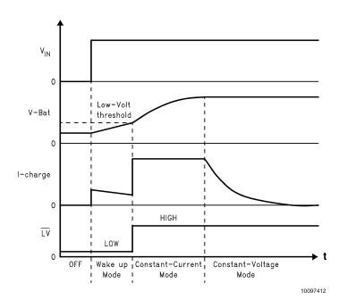
FIGURE 3. Typical Charge Cycle with Low-Voltage Detection Enabled.
