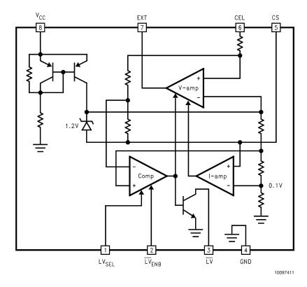
FIGURE 1. LM3622 Simplified Block Diagram
