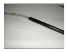
Finally, connect the one end of the flexible tubing to the pen. Make sure that the other end of the pen is sealed. If not, find a way to seal it so that no air can come out.
