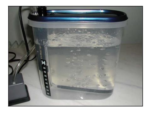
You can put the pump on the top of the container to avoid corrosive liquids enter the device and generally keep things cleaner.
