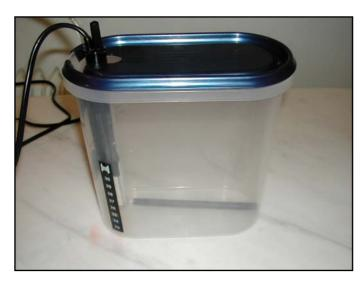
Place the heater on its base and cut the necessary openings on the lid so it can close without blocking the heater and the flexible tubing. Yes, you have finished! Fill with water, pour in your favorite enchant (ferric chloride of ammonium persulphate) and ENJOY PCBing!!! ©
