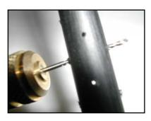
drilled one hole per cm of pen length in the longitudinal direction and replicated this pattern four times along the circumference of the pen.
