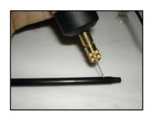
Prepare the bubbler. Use your favourite drill (yes, the one that you drill PCB holes with!) and fill the pen body (remove the ink tube of course first) with holes. I
