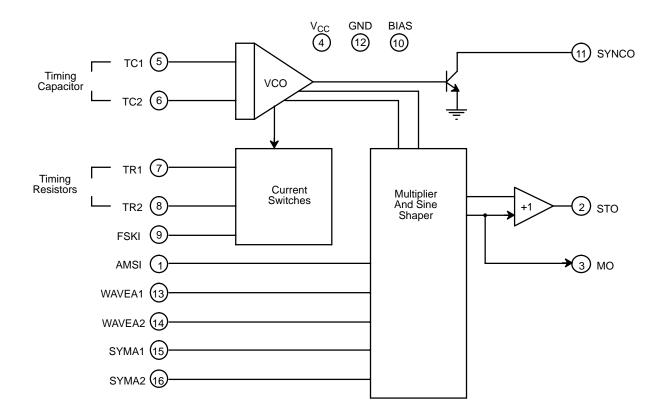
Figure 1. XR-2206 Block Diagram
