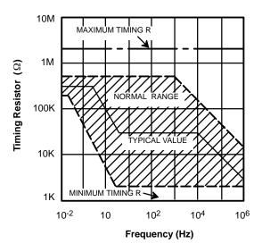
Figure 5. R versus Oscillation Frequency.
