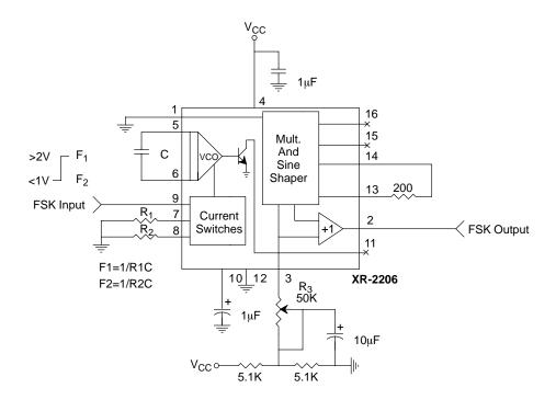
Figure 13. Sinusoidal FSK Generator
