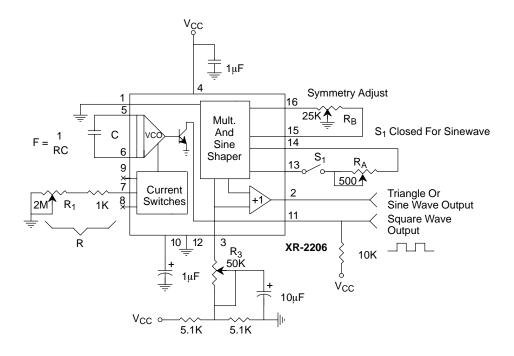
Figure 12. Circuit for Sine Wave Generation with Minimum Harmonic Distortion. (R<sub>3</sub> Determines Output Swing - See *Figure 3*)
