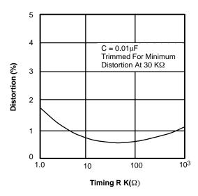
Figure 7. Trimmed Distortion versus Timing Resistor.
