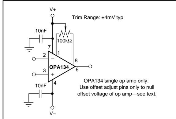
FIGURE 1. OPA134 Offset Voltage Trim Circuit.
