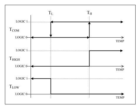
Figure 5. THERMOSTAT OUTPUT OPERATION
