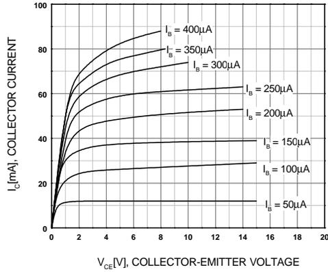
Figure 1. Static Characteristic
